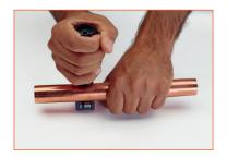
1) **Cut the pipes using suitable tools** that will avoid the risk of buckling. The use of hacksaws and disc grinding wheels are not recommended.
