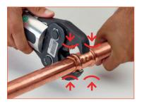
7) Once pressed, the fitting guarantees both the stiffness of the whole system and the perfect tightness of the O-rings. Connections are now no longer divisible, and they resist against high stress. We recommend the periodical maintenance of the jaws, using a degreasing product.
