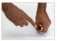
3) Check the correct position of the O-ring inside the toroidal chamber and lubricate it with water and soap. Do not use oil or grease at all.
